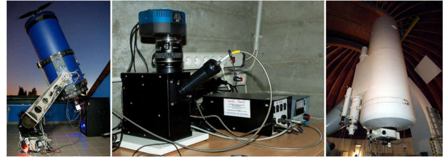
Figure 1. Left: The 0.5m RC telescope of GAO used exclusively for spectroscopic observations. Center: The eShel echelle spectrograph and its accessories: the QSI 532ws CCD camera and the ThAr unit with its power supply box in a thermally isolated concrete room below the 0.5m RC telescope at GAO. Right: 1m RCC telescope of PO.
