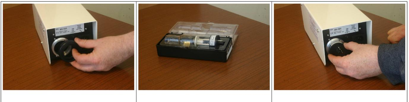
*Fig: installing the Thorium-Argon lamp inside the calibration unit*
