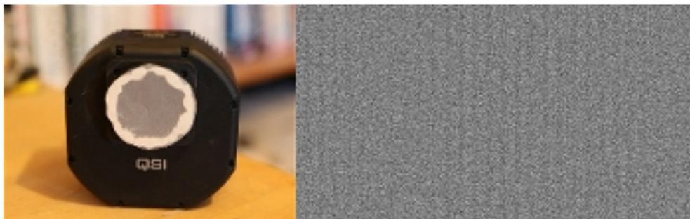
PRNU (Pixel Responsivity Non Uniformity) is acquired with the CCD camera alone, detached from the spectrograph. Cover the entrance with a light diffuser (several layers of a diffuse paper for exemple) in front of a uniform screen (a white wall for exemple), slightly enlighten. Several individual exposures (usually between 0.1 sec and 1 sec). The result should be an uniform (more or less) « flat » frame with intensity level around 1/3rd of the overall dynamic.
