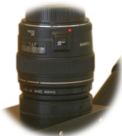
Ensure this is well secured with the three screws on the adapter in between, but note that you will have to rotate the lens once the CCD camera is setup to properly orientate the spectrum on the image. Good alignment is critical for spectra processing.
