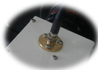
If the spot is not round but has a « comet » type shape, use the two screws close to the power cable connector to adjust the position of the reflective mirror inside the guiding unit.
