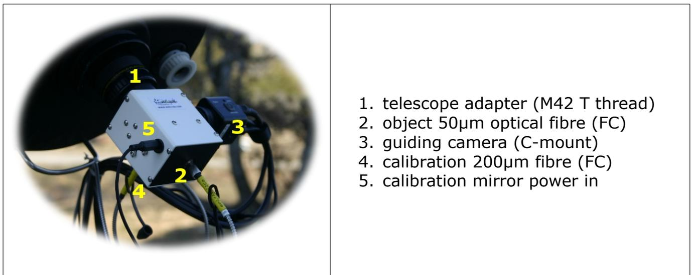
First, a mirror reflects the telescope sky field into a guiding camera. This helps to center the object using a C-mount guiding camera. If you have a CS-mount, use a CS/C extender for optimal performance.
