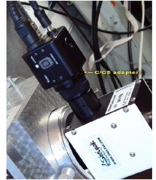
Connect the remote controller on the camera, the video cable, the grabber (install the grabber software before connecting it; follow the on-screen instruction of the grabber software). Connect the camera on the guiding port and power on.
