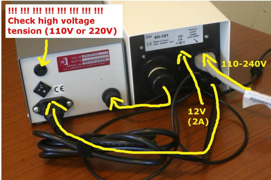
Fig: high voltage power supply and calibration unit
