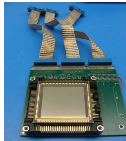
AQUARIUS detector on PCB also shown are woven manganin ribbon cables
