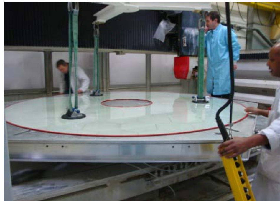
2.6m glass shell, 2 mm thick at SAGEM
