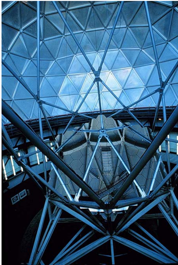
View of telescope with all 91 hexagonal mirrors installed.
