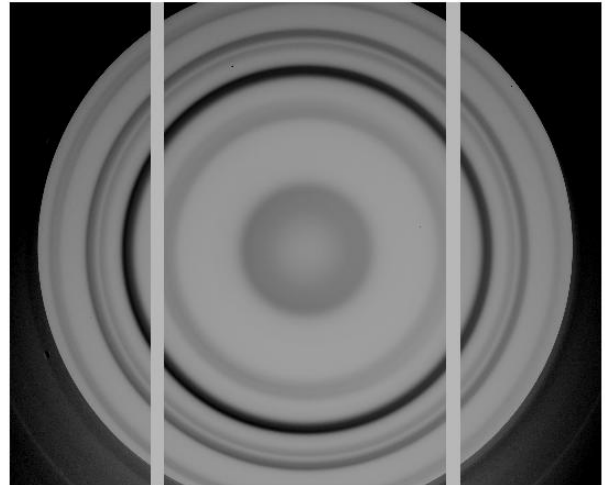
Figure 14b: Same as fig. 14a, but with the High Resolution etalon and same filter. Multiple rings arise from different lines falling within the filter bandpass.
