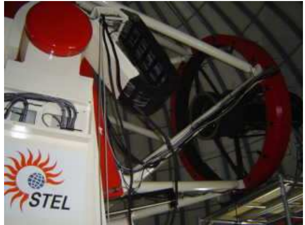
1.8-m MOA telescope, with 500mm diameter prime focus corrector.
