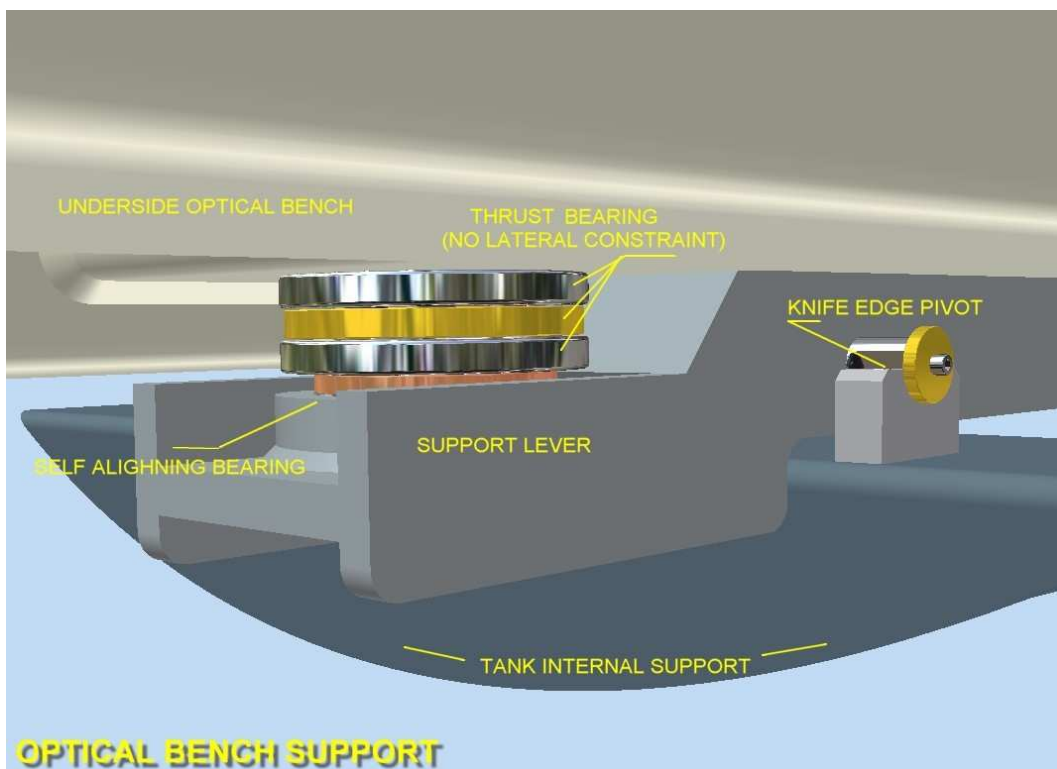
Figure 5: The optical bench support (from underneath) showing thrust bearing, with self-aligning bearing, support lever and knife edge pivot point.
