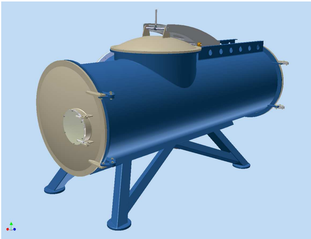
Figure 4: Final tank design showing lever and hinge arrangements for lids.
