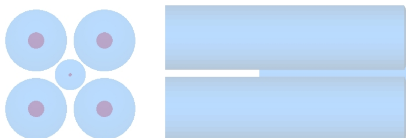
Figure 13: Schematic plan (left) and elevation (right) of the direct injection micro-lenses. The plan shows the grouping of the four 500 \mu\text{m} fibres and their micro-lenses with a fifth 100 \mu\text{m} fibre and smaller micro-lens in the middle.
