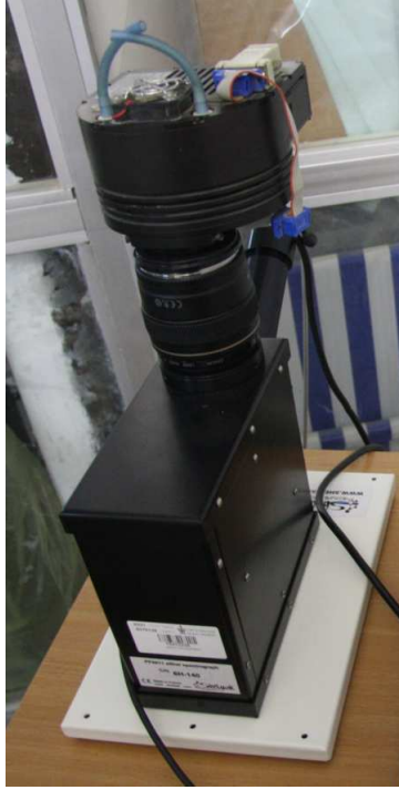
Figure 6.3: The spectrograph unit. The SBIG ST-10ME CCD camera is on top of the CANON objective lens. The object fiber connects to it from the back.
