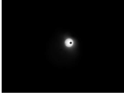
Figure 6.6: Image of the pinhole as it is lit by the ThAr lamp (SBIG St-i CCD Image)
