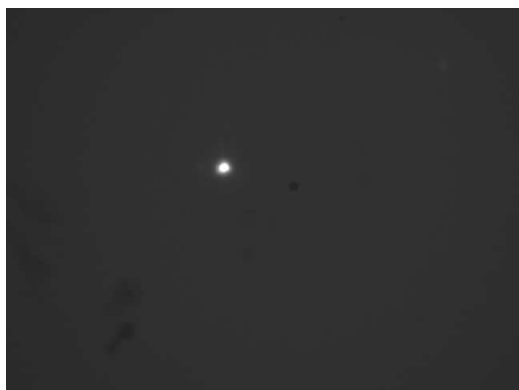
Figure 6.8: Image of the ST-i CCD with a star and pinhole after focusing.
