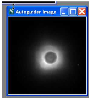
Figure 6.10: Autoguider on a star with the pinhole in the middle.
