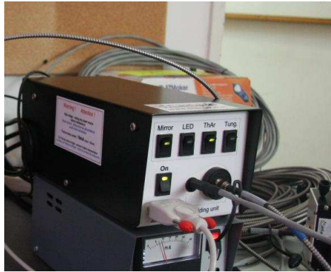
Figure 6.2: The calibration unit with the switches that control the calibration sources and the FIGU mirror
